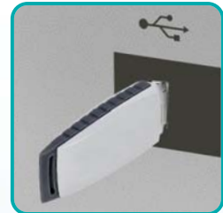
USB port for use with flash drives to record data
